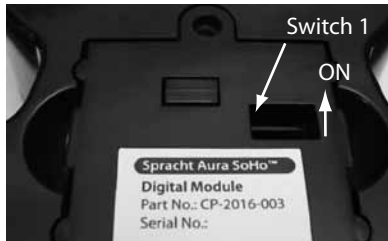
Location of Switches
